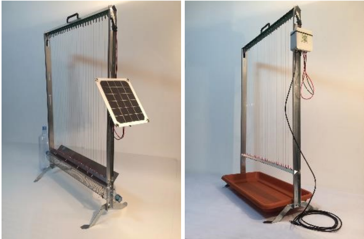
Figure 1: Spanish Arpa Electrica's by SANVE (Sanve.weebly.com) Dry arpa left and wet arpa right). Photograph courtesy of SANVE
