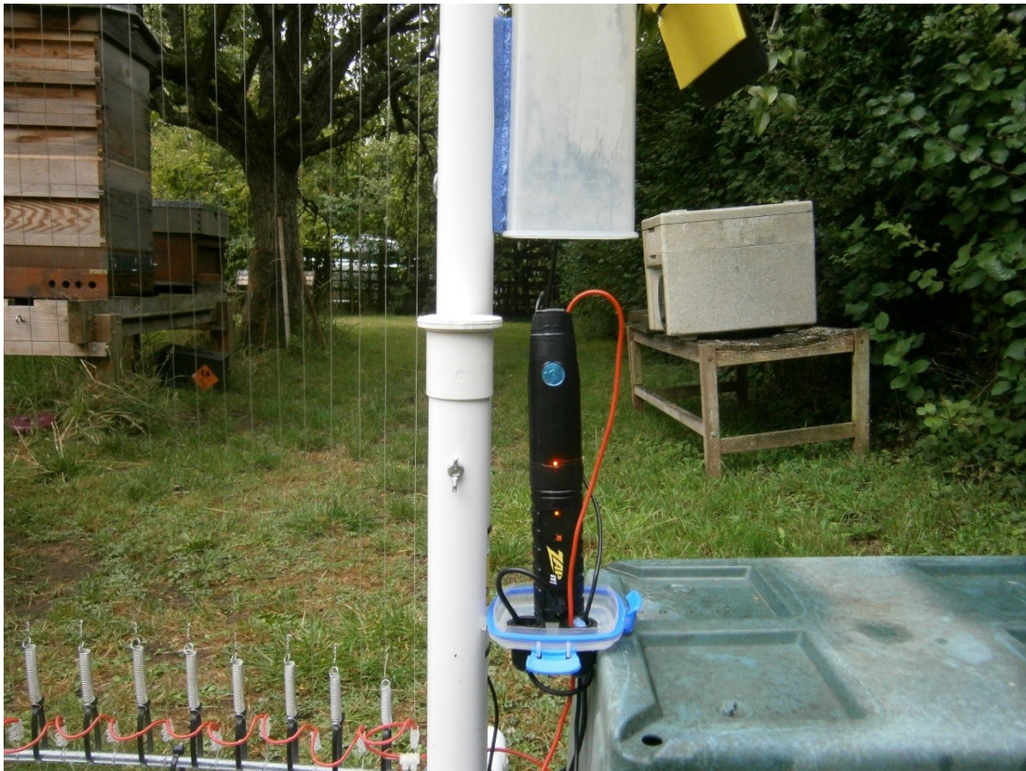
Figure 7: Homemade HV power unit. Photograph by Andrew Durham Note: This was an early model that showed up the problem with using the threaded rods as electrical conductors. The red copper wires were a solution to the problem but nowadays I would not use copper wires for this purpose because they corrode. I would use stainless steel links as shown in figure 5 above.
