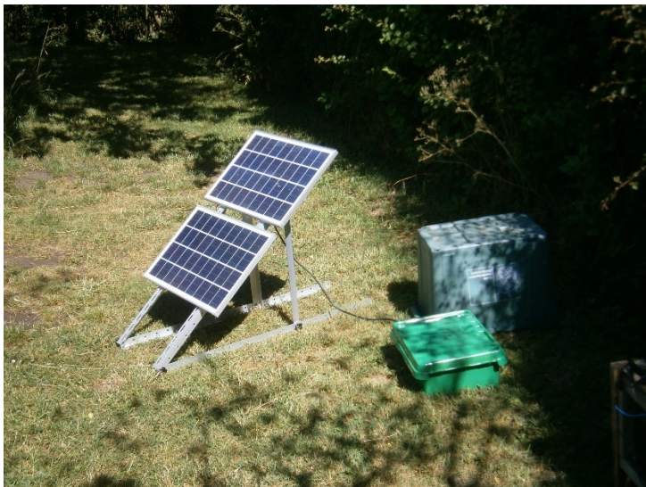
Figure 8: Two ECO-WORTHY 25 Watt 12 Volt Polycrystalline Solar Panel Modules providing solar power – Photograph by Andrew Durham (Note: One panel should suffice; a second can easily be added if required)
